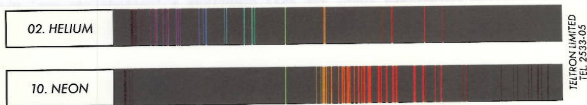
FIGURE 02 : OPTICAL SPECTRA OF HELIUM AND NEON
